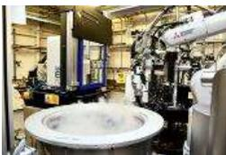
*The experimental hutch of Diamond's beamline I04-1 where XChem experiments are measured, showing the detector and BART sample changing robot that can hold 592 separate samples.*
